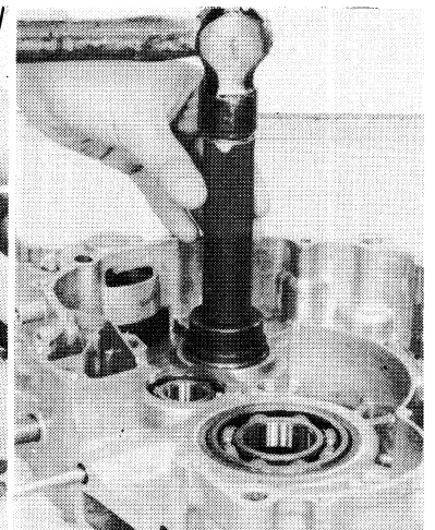
BEARING REMOVER, 17 mm 07936-3710300 REMOVER HANDLE 07936-3710100
