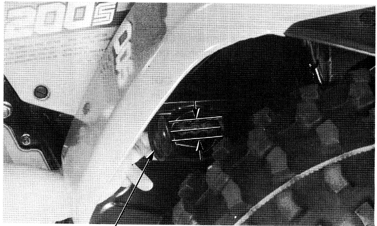
INSPECTION HOLE CAP
